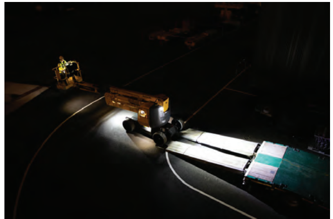
ALL IMAGES: Haulotte's new electric articulating booms, Sigma 16 and Sigma 16 Pro, have a working height of up to 16 m.
