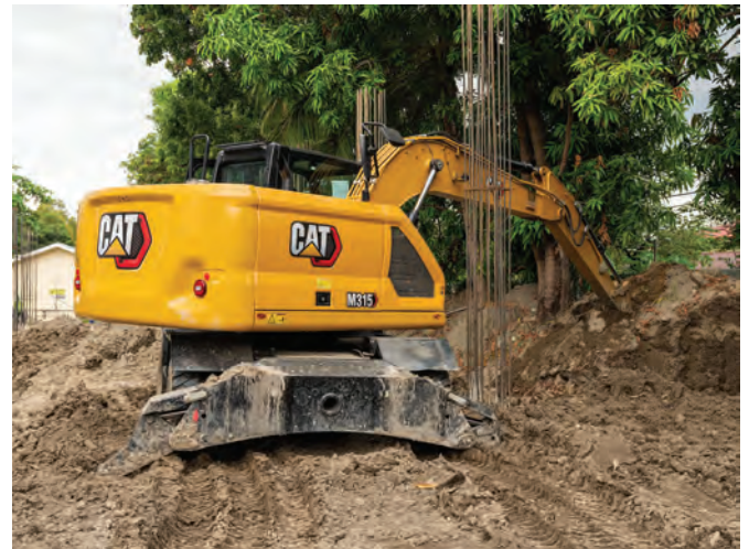
ABOVE AND BELOW: The Cat M315 excavator offers up to 14% more swing torque and technology options to boost productivity. The machine can travel between sites easily with travel speeds of up to 37 km/hr.
