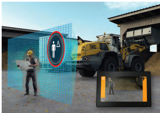
The Liebherr brake assistant automatically decelerates the wheel loader the moment the active personnel detection identifies a source of danger in the rear area.
