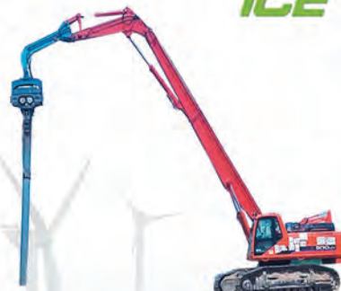
Excavator Vibro Hammer
