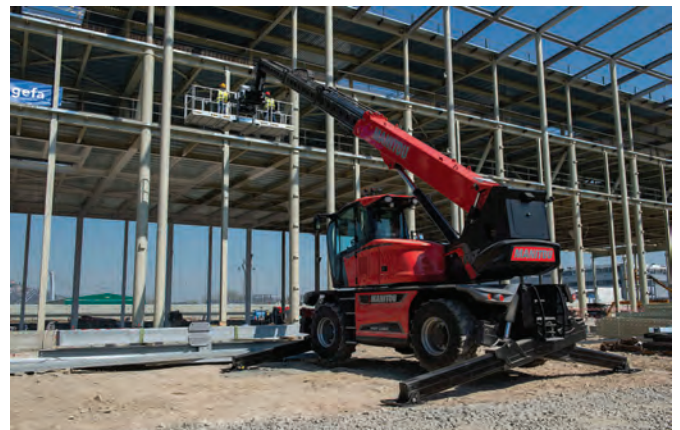
ALL IMAGES: The redesigned MRT rotating telehandlers from Manitou, comprising the Vision and Vision+ ranges, are available for the global market.
