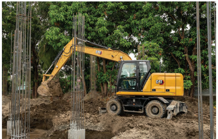
ABOVE AND BELOW: The Cat M315 excavator offers up to 14% more swing torque and technology options to boost productivity. The machine can travel between sites easily with travel speeds of up to 37 km/hr.
