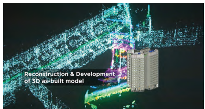
ABOVE: By using drone fleets and robotics systems equipped with LiDAR laser scanning technology, a 3D model of the construction site can be progressively built up as construction progresses.
